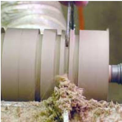
Use the parting tool and calipers to size down to the required diameters. The calipers float of the wood; if pressure is applied, the calipers may spread.
