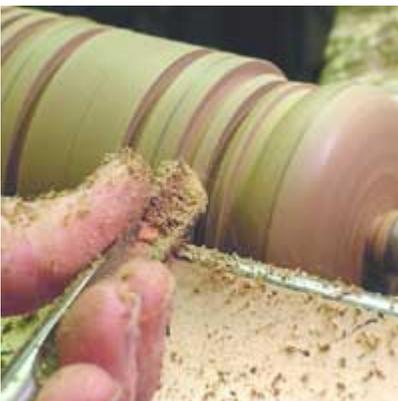
Starting to cut the cove with the gouge on its side and bevel pointed where the cut will end at the bottom center. Cutting a cove requires moving the gouge handle in a long arc and rotating the handle at the same time.
