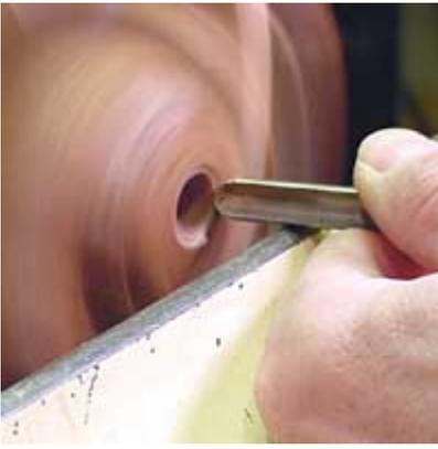
The opening for the handle is a convex shape with two high and two low areas. I chamfer the opening with a gouge to allow the round shape at the top of the handle to seat all the way down to the low spots.
