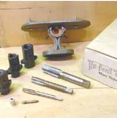
The Beall wood threading kit. Three sizes of taps and inserts for the router fixture (1/2", 3/4" and 1"), a double ended cutting bit and a pilot bushing to align the fixture on the router.
