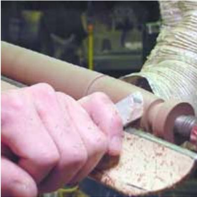
Start shaping the handle from the tailstock and work back to the headstock end.
