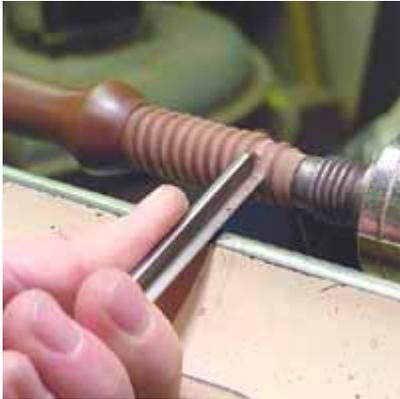
I grip the end of the handle in the chuck with foam for padding. I can now do all the shaping and cut to length. Turn away the threads to match the end of the tap.
