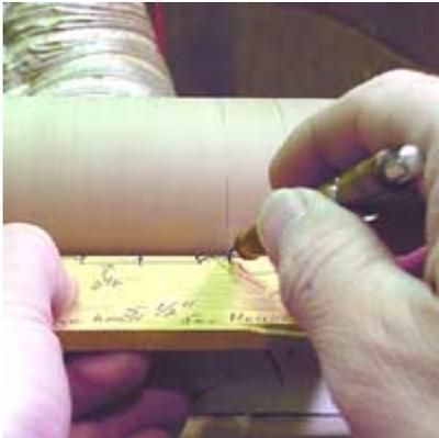
With the lathe on transfer the layout points to the blank. Each point on the storyboard that needs to be marked precisely has a small V notch for the pencil to rest in.
