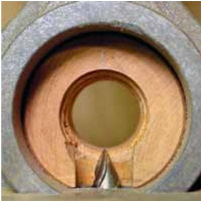
The fixture for threading the handle, ready to go with the bit height checked on a scrap dowel. I made the die from a piece of boxwood. If the bit is not set deep enough to make the full thread the handle will not turn and the height will need adjusted.
