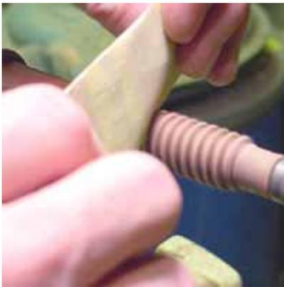
Sand the threads with fine sand paper to remove the fuzzed up grain. With the lathe running, sand each side and the tops of the threads.
