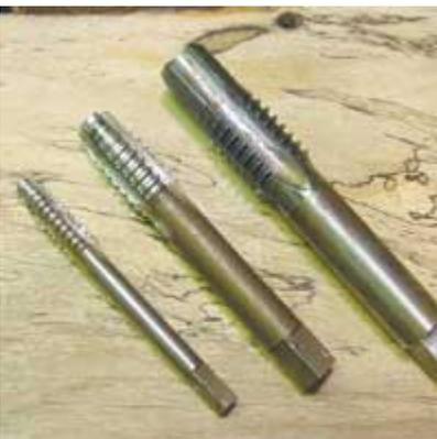
The taps have a long pilot section on the end that I have cut off to be able to thread deeper in a blind hole. The largest tap still has the long pilot end.
