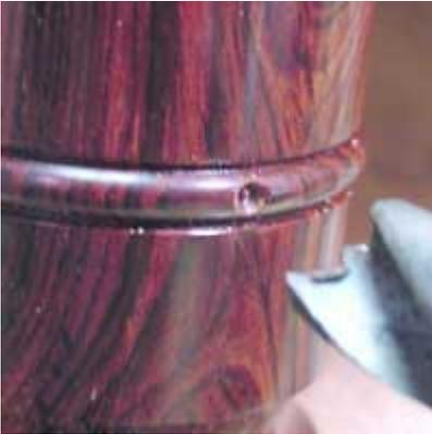
You will find out if you have turned a gavel head exactly the same measurement on each half if you add an element like this small bead in the center. You will also find out if you lathe centers align when you start to drill.
