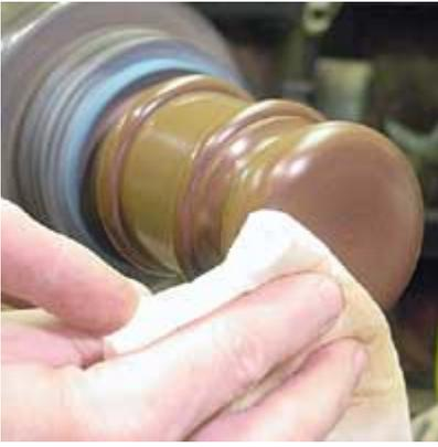
Apply a finish of your choice. I use a three-part finish made of equal parts of denatured alcohol, boiled linseed oil and clear shellac. Lacquer and other surface build finishes look bad on the faces after a few years of use.
