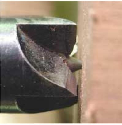
To quickly center, the blank I roughly eye the center and stick the spur point into the wood enough to hold it. Bring the tailstock in to hold the other end and rotate the blank to check centering. If not I move the point to another point and check again until centered. I cut all my blanks slightly oversize so I do not have to center perfect to keep the finished diameter I want. Once centered tighten the tailstock to engage the spurs on the center.
