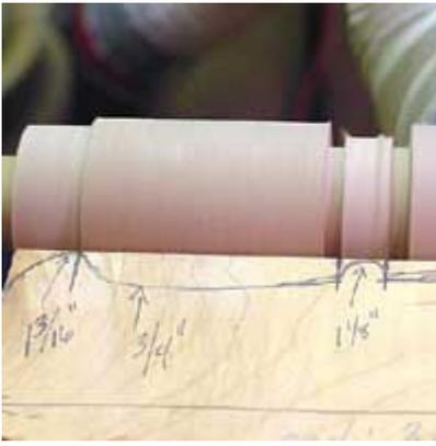
To the left I have made my sizing cuts to align with the point where the cuts need to start as a reference. One side is half a bead and the other half is half a cove.
