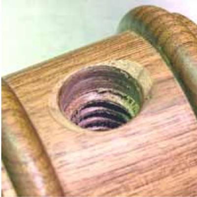
The finished threaded hole with the counter bore and chamfer.
