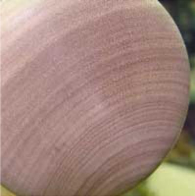
The face of the gavel is clean cut. Do not leave spur or tailstock center marks in the gavel faces. The gavel samples shown to me at the State Capitol had them still in the faces and a screw through the top of the head to hold the handle in place.
