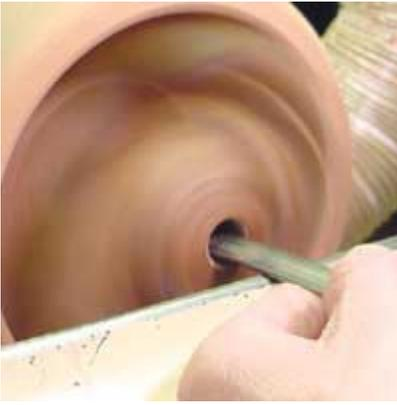
If I wanted to make a blinded wedged tenon as the head attachment method I would now make the hole tapered from narrow at the opening to wide inside with the long point of the skew or a scraper ground for the purpose.
