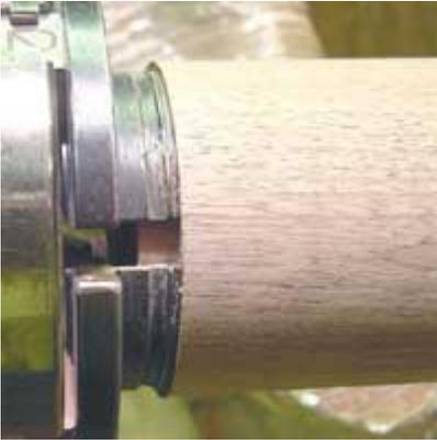
The tenon seated firmly against the chuck jaws so the largest diameter area gives good lateral support while turning an unsupported spindle.
