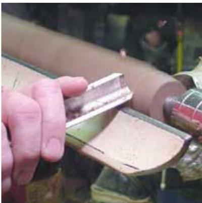
Start roughing to round at the tailstock end and work back toward the headstock.
