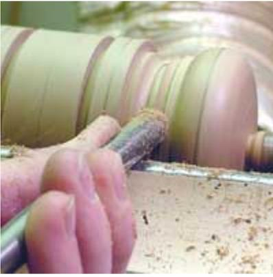
Cut the other side of the cove the same way. Work the cove from each side until you have one continuous curve.
