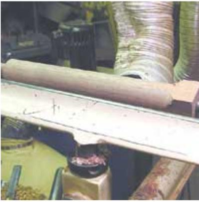
Reverse the handle blank and grip the thread tenon in the chuck. Turn the square section to round that was in the chuck jaws.
