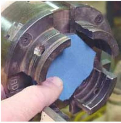
To hold the finished end of the head I use my Oneway collet chuck jaws without the aluminum inserts. I have ground the sharp edges off the inside of each jaw so they do not mar the surface. Here I am putting a piece of foam in the back of the chuck to protect the finished face.
