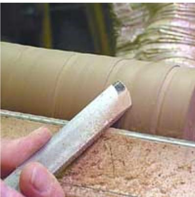
Turn the whole blank down to the sized areas. Cut the surface cleanly because the tops of the beads and ends are at this level. The cylinder needs to be a consistent diameter all the way across. I do not want one end of the gavel larger than the other one.
