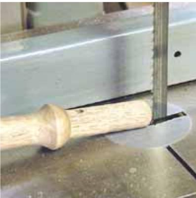
I split the handle on the band saw with the stop hole vertical and the tenon riding on the table.
