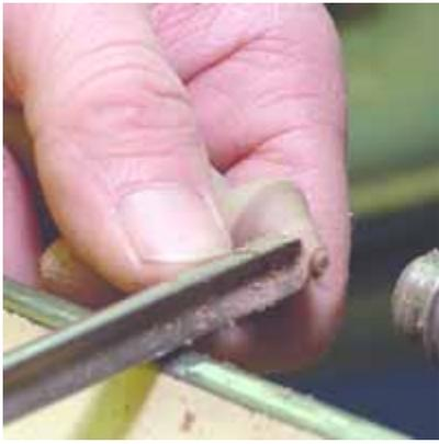
With everything turned the end of the handle can now be finished with the tailstock backed off. Lightly grip the rotating handle in your fingers and shape the end.
