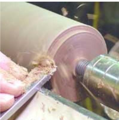
I am using a peeling cut with the skew on its side to form a tenon for the chuck.
