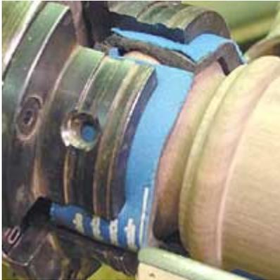
I use a piece of foam from a computer mouse pad to cushion the finished end.
