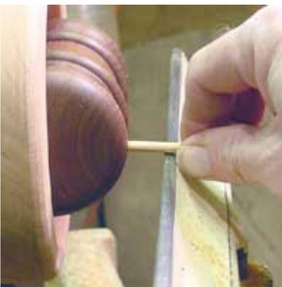
Rotate each end of the head past a fixed point and adjust the head until both are the same. Tap with your hand or soft face mallet to adjust.
