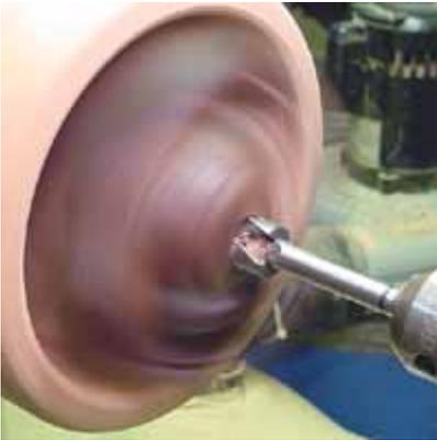
The threaded hand has a short section of straight shaft about  $\frac{3}{8}$ " long that I counter bore for at the start of the hole.
