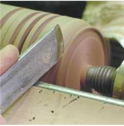
I start turning at the tailstock end and work my way toward the headstock.
