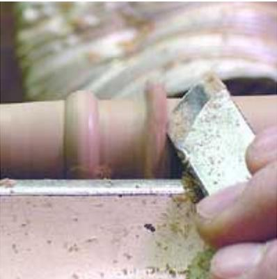
Using the skew to bring the handle up to the bead for a sharp transition. Do not take too deep a cut with the point or the grain could tear out. The cut in front of my point is a thin rolled continuous ring of wood. I want the point to come up to the bead side and stop, not undercut the bead.
