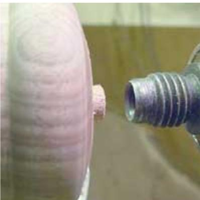
The 7/16" tenon and the tapered inside of the live center. I do not use a center point in my live center except to hold a pen mandrel end. All other turning I do with the cup as a contact area only.
