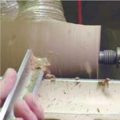
Start roughing the blank from either end, not in the middle, and cut back across the blank until round.
