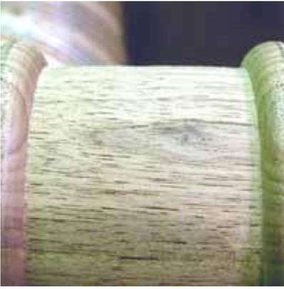
The finish turned center of the head. Surface finish straight from the tool and pencil lines intact.
