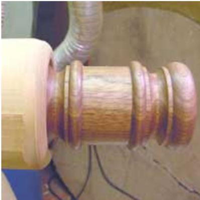
Another way to hold the finished face. Turn a recess in a waste block mounted on a faceplate. If you are turning several heads, measure them all and start with the smallest one then enlarge the jam chuck to fit each larger end.
