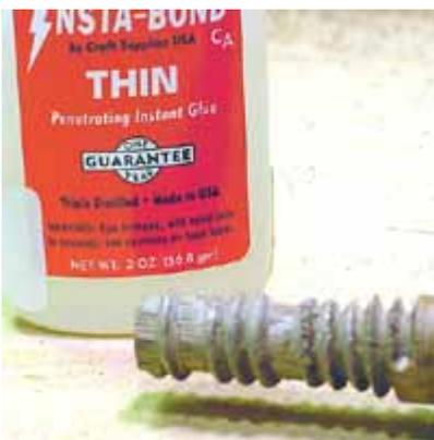
Do not use glue on the thread area before routing the threads. The broken threads to the left are the result. I thought that hardening the top edges of the threads with thin glue before routing would make them less likely to chip and break. I was wrong. The glue soaked threads broke off and jammed inside the die.
