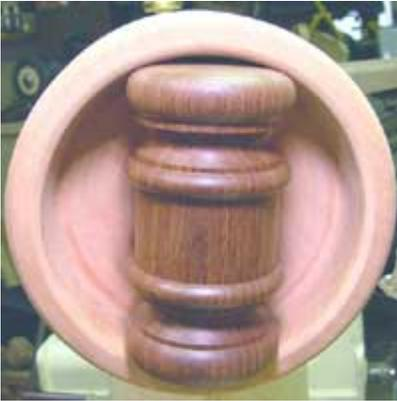
I saw a video by Dennis White of England turning a gavel and it showed how he drilled the head perfectly centered in a jam chuck like this one. It looks bad to have the handle angled to the head or offset to one side when you look at the gavel from the end. With this method, all you have to do is drill and the handle aligns perfectly with the head.
