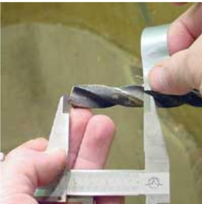
Now transfer the depth measurement to the drill bit. I use a piece of tape to mark the drill.
