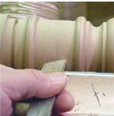
Remove the excess wood from between the beads. I use the skew on its side to flatten this area working from side to side. This is just a light cut that removes any ridges. It leaves a surface that sands well and does not tear the grain.
