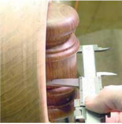
Measure the diameter where the head will be drilled and subtract about  $\frac{1}{2}$ " so the drill does not go all the way through the head. If this was a carving mallet or other type shop mallet I would not mind the handle going all the way through but for a gavel I think it is not good practice.
