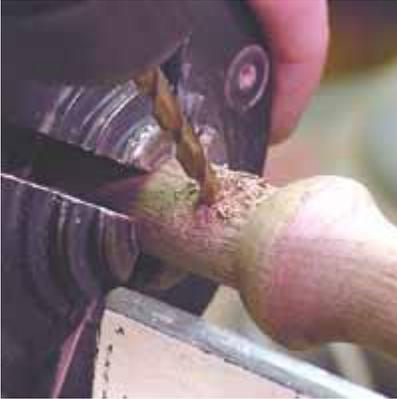
Drill a hole through the handle of the tenon as a stop hole for the saw cut.
