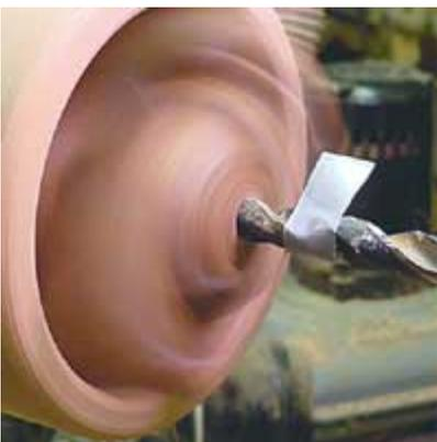
Turn the lathe on and drill to the depth mark. I usually drill at a speed around 300 rpm.
