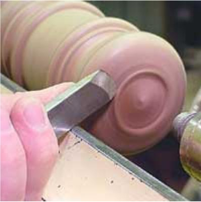
With all the elements turned, I can now slide the tailstock back and finish the outboard face. I use the skew long point for this. Endgrain surfaces are hard to sand torn grain areas out of so make sure there are none. A sharp tool is essential for this.
