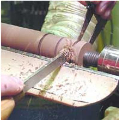
Set the calipers and make a few sizing cuts as reference to turn down to.
