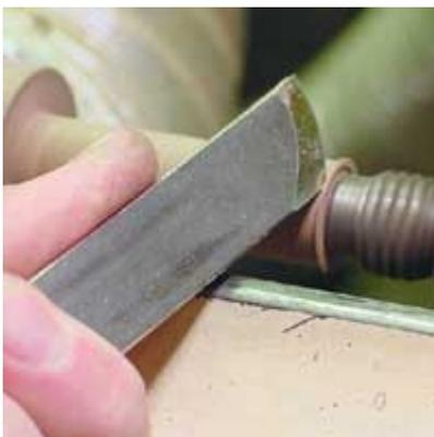
Chamfer the end of the spindle to make starting the thread cutting easier.
