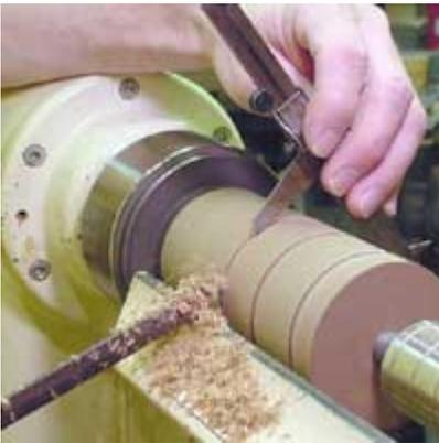
Sizing the blank to slightly over the desired diameter. When I say slightly over, I mean about  $1/64$ ". Sanding will reduce the diameter by a small amount later.
