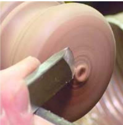
The center of the wood moves at fewer feet per revolution speed so the cut has to slow as it nears the center also.
