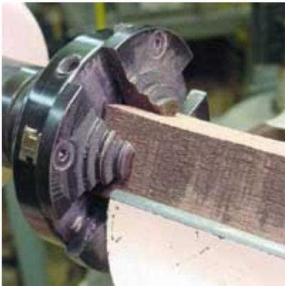
I use my Nova chuck with the number 1 jaws to grip the square for the handle. Center the tailstock end of the blank and tighten the jaws.
