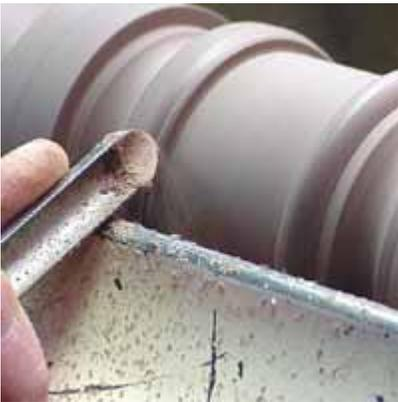
Shape the beads and leave the pencil marks intact. Many turners keep trying to cut the perfect bead by going back to the center and starting the cut again. Each time this happens the diameter of the bead shrinks. Avoid this by starting a good round shape with the first cut and repeating it in steps until the side is finished.
