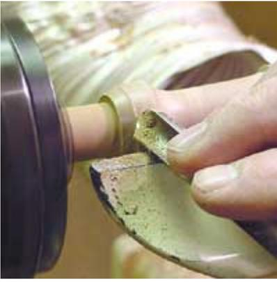
Round the top shape to the thread straight section.
