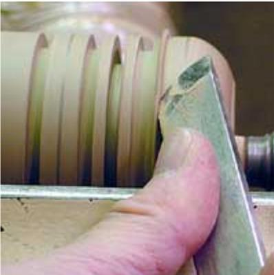
You can see a pencil line that is the high point on the end and another to the left, the center of the bead. Do not turn the pencil lines away and you will not be reducing the diameter.
