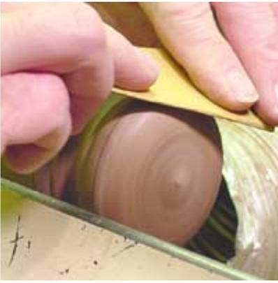
Sand the finish turned areas. I usually start with 180 grit and work up to 400 or 600 grit depending on the wood. I often apply a finish now to protect the wood from handling in further operations.
